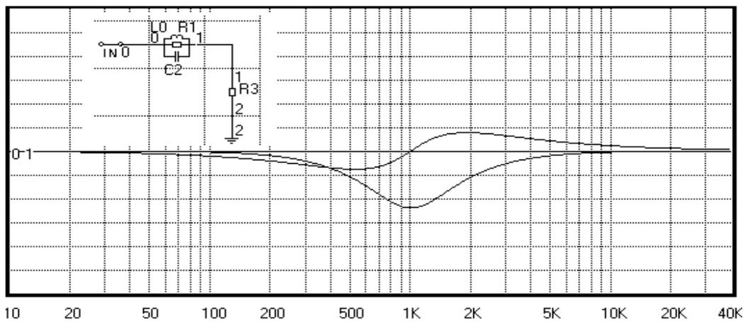
Figure 6. Trap circuit that has similar response to overlapped L-R crossover. Scale: 3db/division.
