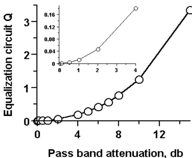
Figure 11. Q of required equalization circuit.
