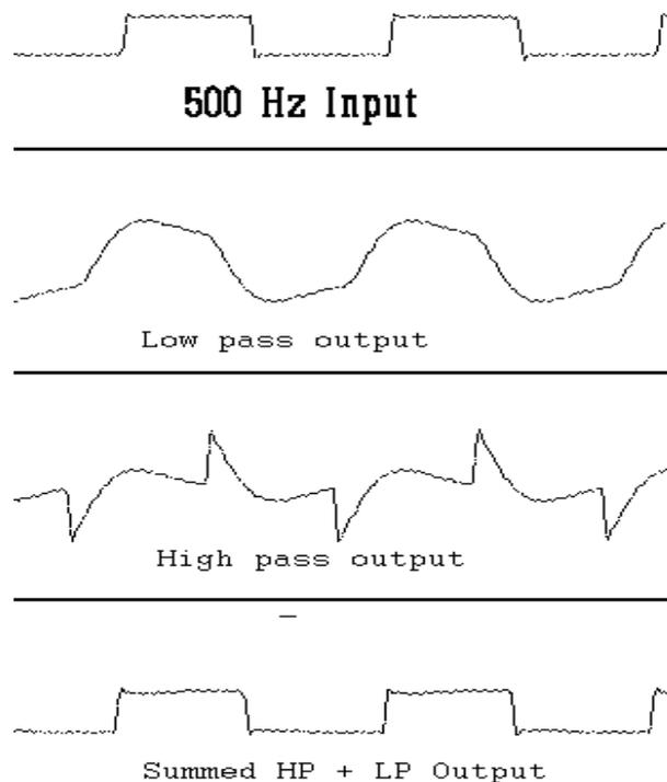
Figure 17. Experimental result for a 500 Hz square wave
