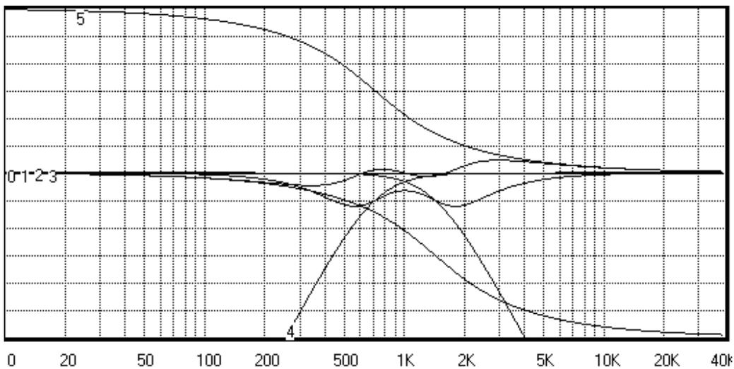
Figure 3. Summed 2<sup>nd</sup> order overlapped Butterworth crossover at 1k Hz following Lipshitz and Vanderkooy [2]. Overlap parameter = 2. Scale: 3db/division
