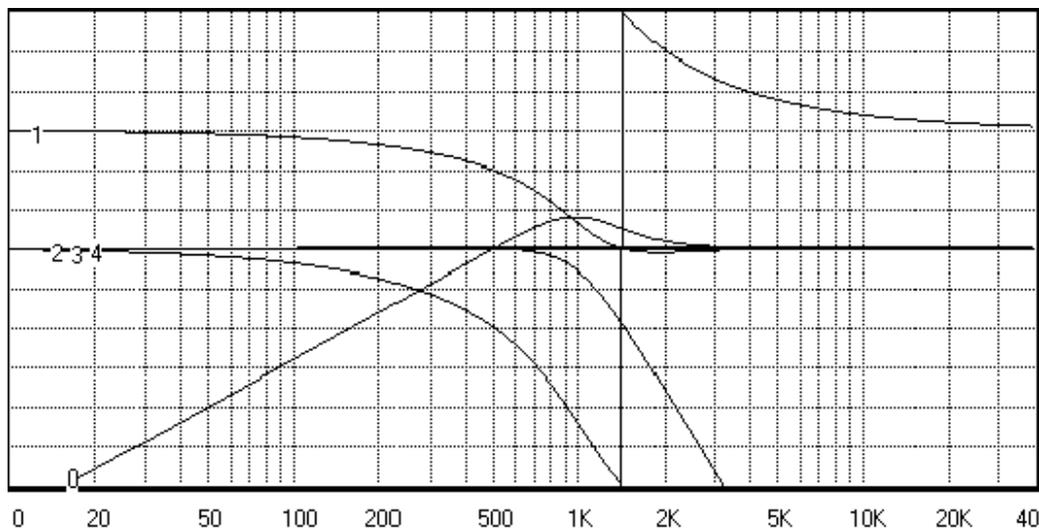
Figure 1. Constant voltage crossover HP and LP sections employing a 3<sup>rd</sup> order Butterworth low-pass filter. 0 - HP amplitude response, 1-HP phase response. Scale: 5db/division
