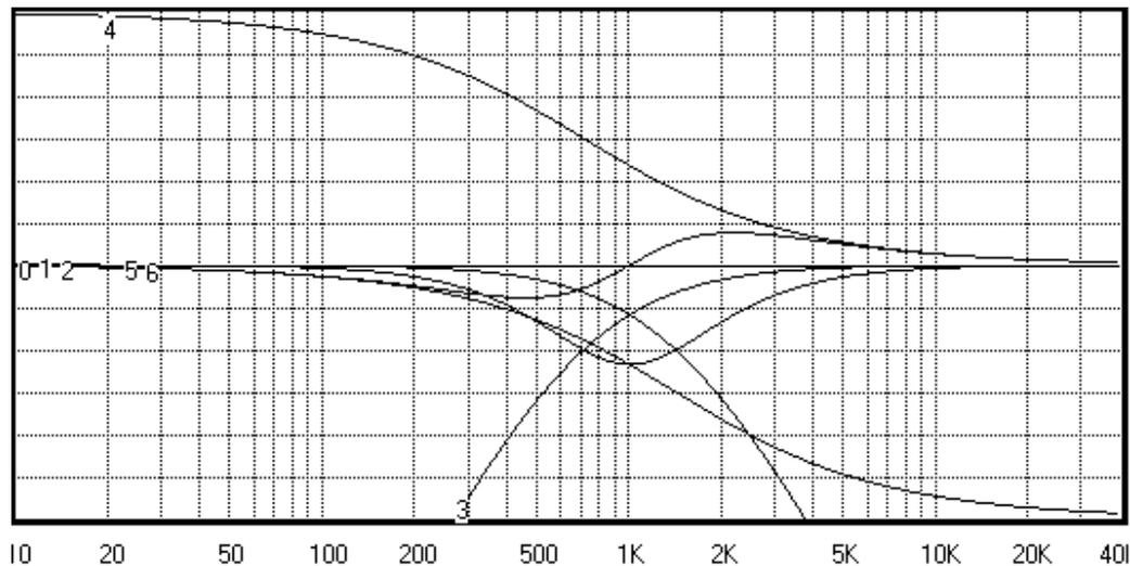
Figure 4. Summed 2<sup>nd</sup> order overlapped Linkwitz-Riley crossover at 1k Hz following Lipshitz and Vanderkooy [2]. Overlap parameter = 2. Scale: 3db/division
