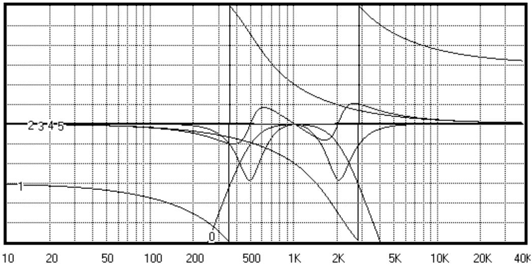
Figure 5. Summed 3<sup>rd</sup> order overlapped Butterworth crossover at 1k Hz following Lipshitz and Vanderkooy [2]. Overlap parameter = 4. Scale: 3db/division.
