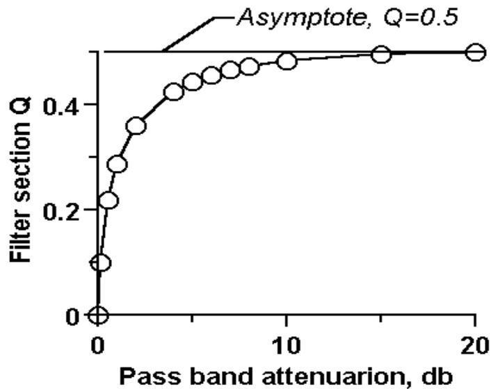
Figure 9. Filter section Q vs. pass band attenuation.
