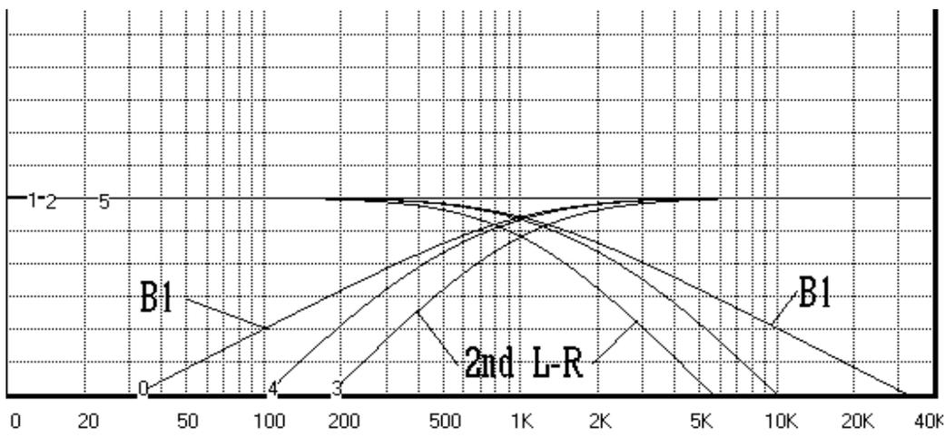
Figure 15. Comparison of 2<sup>nd</sup> order L-R, 1<sup>st</sup> order Butterworth and present HP and LP filter amplitude responses. Scale: 5 db/division.
