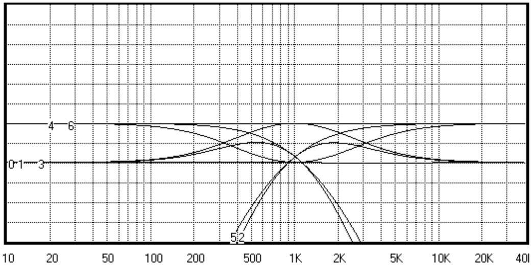
Figure 12. Amplitude response of HP and LP filter sections with and without equalization, summed response with and without equalization, and the equalization response. Scale: 2 db/division.
