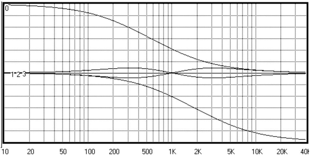
Figure 13. Phase response of unequaled HP and LP sections, summed unequaled phase, and phase of equalization circuit. Scale: 30° per division.
