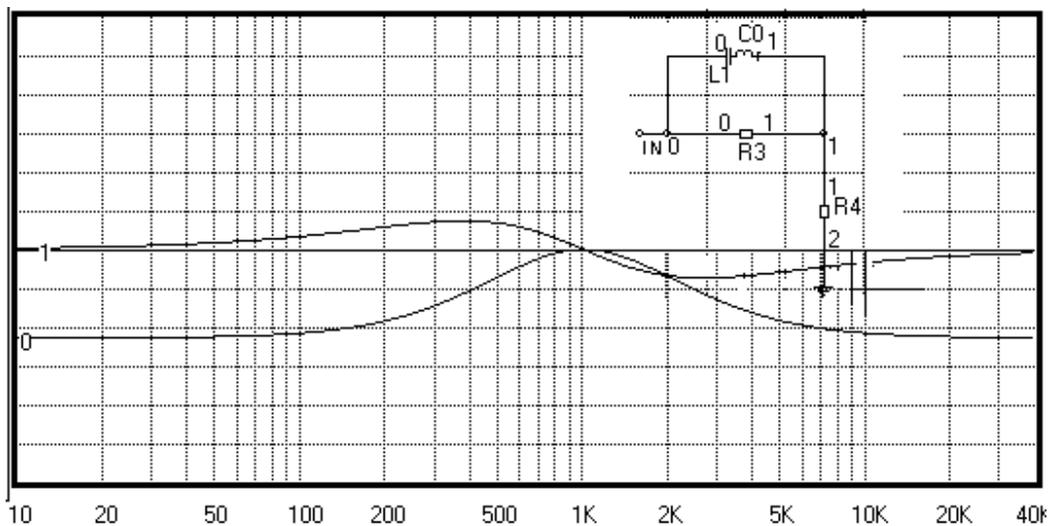
Figure 7. Passive equalization circuit for overlapped 2<sup>nd</sup> order Linkwitz-Riley crossover. Scale: 3db/division.
