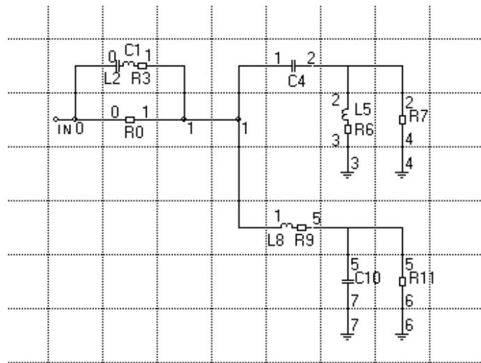
Figure 8. Second order crossover and equalization used in CALSOD optimization.
