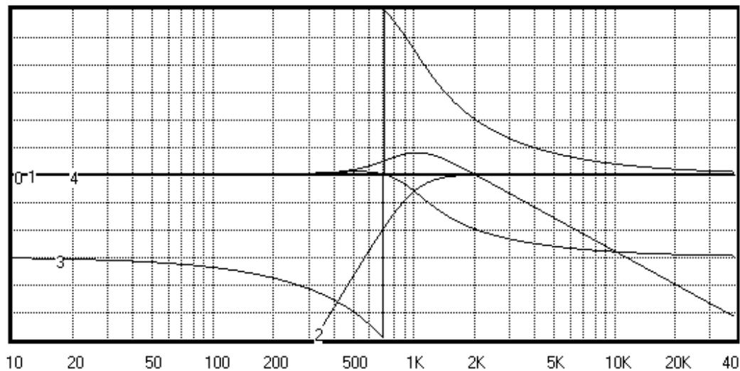
Figure 2. Constant voltage crossover HP and LP sections employing a 3<sup>rd</sup> order Butterworth high-pass filter. Scale: 5db/division
