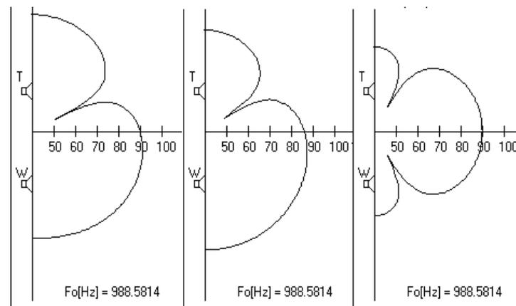
Figure 16. Theoretical vertical polar response at 1K Hz for 1<sup>st</sup> order Butterworth (left), the present 2<sup>nd</sup> order overlapped (center) and 2<sup>nd</sup> order L-R (right) crossovers.
